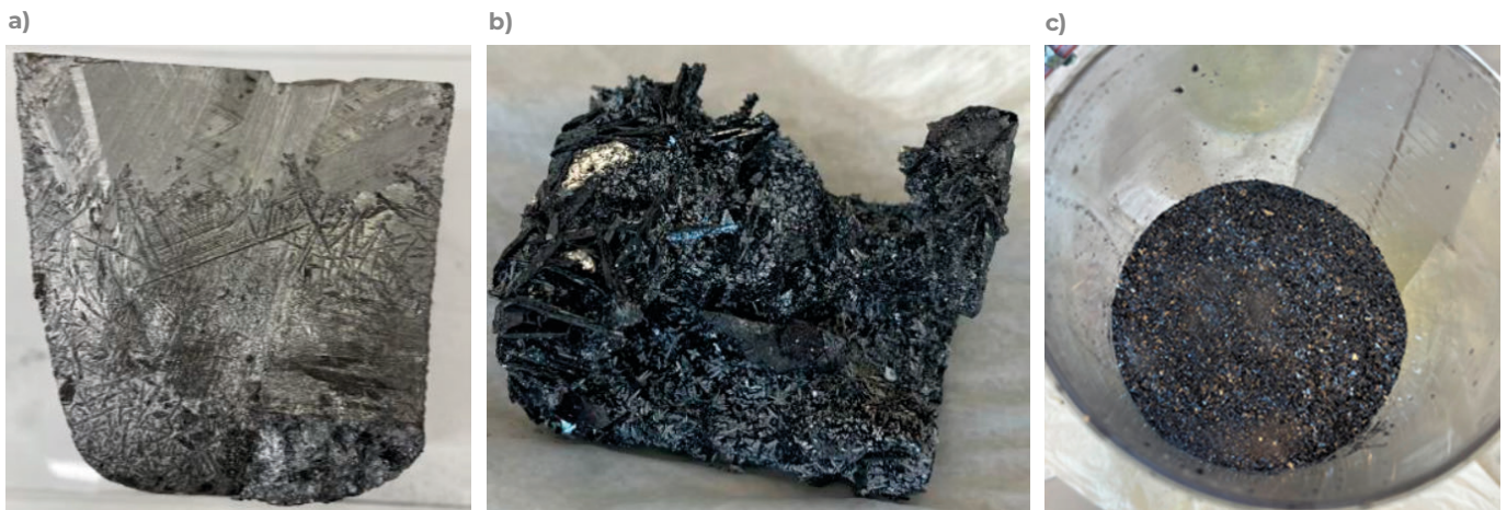
Figure 1 a) Al-Si alloy Si crystals precipitate and form flakes, b) Si flakes resulted from the metallurgical purification, and c) Refined Si particles after acid leaching
